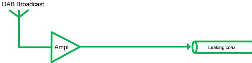
The on-air signal is amplified and feeds a radiation cable inside the tunnel. This provides DAB coverage in the tunnel, and the radiation cable is also used for other frequencies, as FM, VHF, Mobile Network and others.
