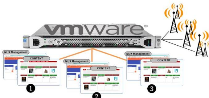
The new system contains a complete system with multiplexers, audio encoder and is installed as fully redundant. The system is provided as virtual machines installed in two separated network locations and uses VMware technology and also contains the Paneda SMART content redundancy switching.
